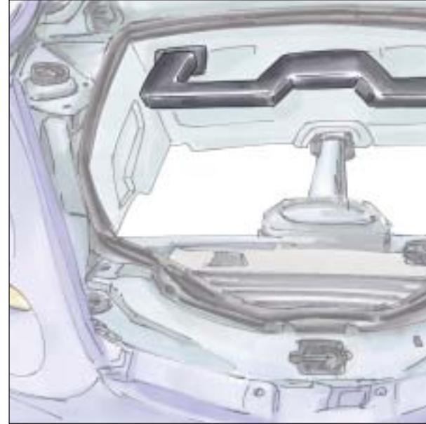
Sealing of welds, bonding of bodywork parts in the engine compartment
