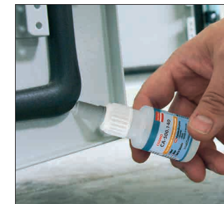
bonding of door seals
