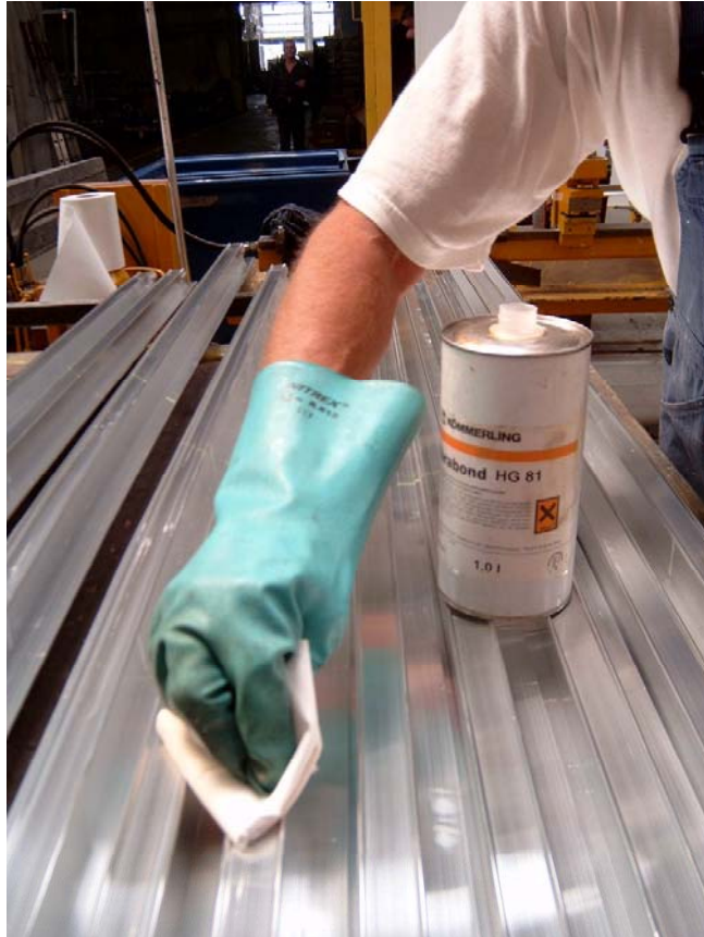
Pretreatment of bonding parts with adhesion promoter Körabond before using 1-part PU or MS
