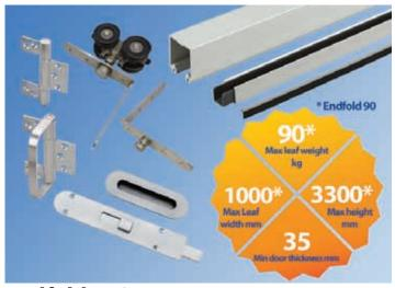
**Endfold 50/90** Folding door system suitable for both residential and commercial applications. Features include nylon wheels with bearings, anodised aluminium track, track & floor mounted pivots and a range of hinges and flush bolts either in a satin stainless or polished gold PVD finish. The 90kg replaces pivots with hinges for greater performance.
